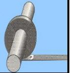
The constant force spring is used for a linear movement and gives an almost constant force at deflection.
